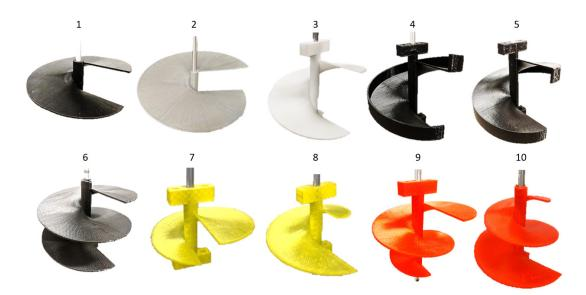
FIGURE 2.2: 3D printed rotors used for experimental tests
