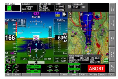
FIGURE 13.3: Multi-function tablet display for in flight vehicle information
