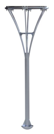
FIGURE 8.8: Individual landing leg attached to nacelle structure
